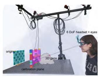
Figure 2. The technical setup to measure 3D gaze inside the tracking volume of approximately 50x50x50cm.
